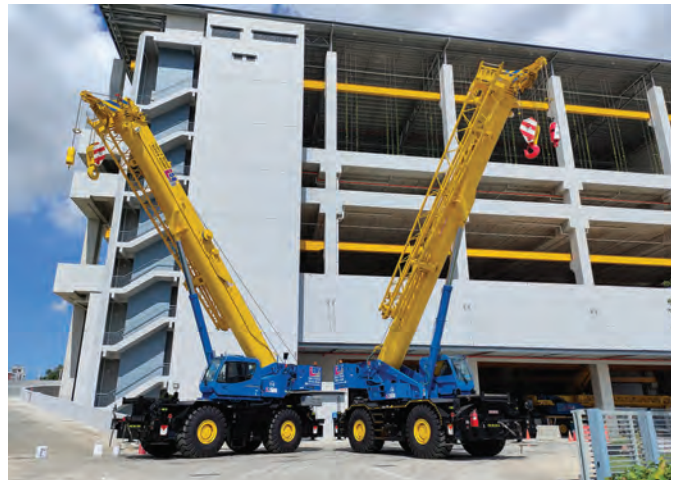
The GR-1000EX-4 rough-terrain cranes have a lifting capacity of 100 t.
