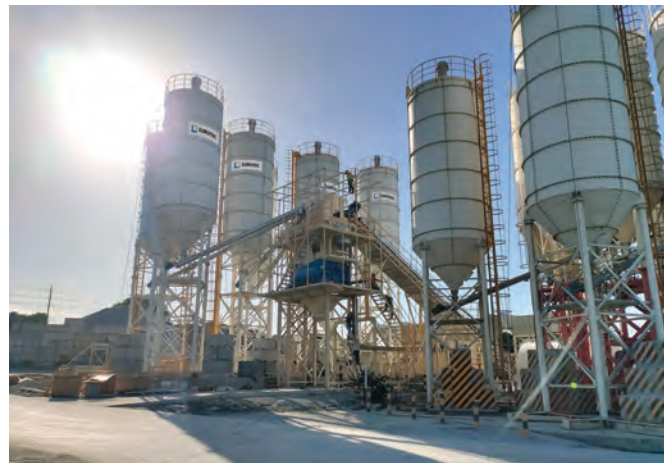
ABOVE: In Batangas, a Eurotec ECO90 plant has been supplying up to 90 cu m/hr of ready-mix concrete for commercial projects.
