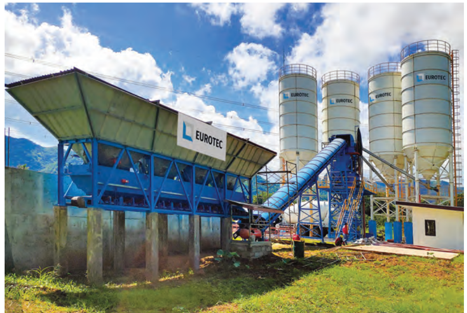
ABOVE: In Batangas, a Eurotec ECO90 plant has been supplying up to 90 cu m/hr of ready-mix concrete for commercial projects.
