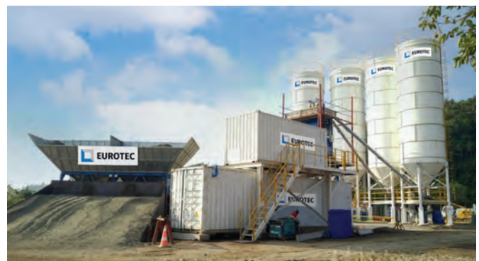
TOP: A Eurotec PTT120 plant produced high-quality concrete for a two-year project at the Manila International Airport. This unit is designed in modules for enhanced portability and easy transportation.
