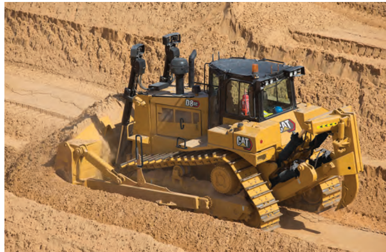
The new Cat D8 GC dozer has 220 kW of nominal net power and an operating weight of 37,557 kg.
